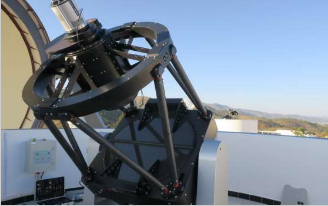
星河科研社聯合德國及奧地利團隊，為中科院雲南基地建造的兩台 0.8 米口徑 f/2.2 主焦廣域巡天望遠鏡。 Two 0.8 meter f/2.2 wide field telescopes for Chinese Academy of Sciences at Yunnan base, co-developed and built by Germany & Austria engineering team and Galaxy Scientific Group .
